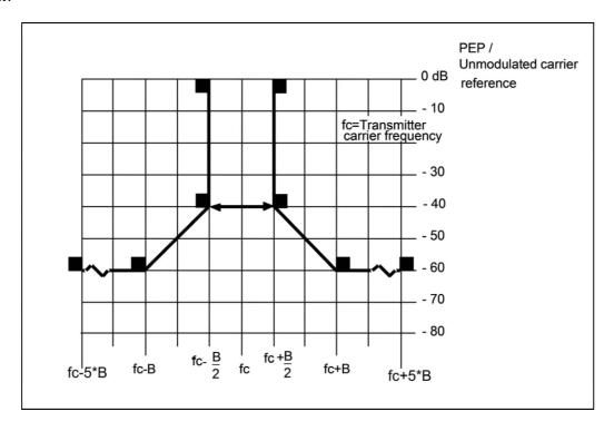
Figure 5: Spectrum mask for digital systems above 2 GHz
