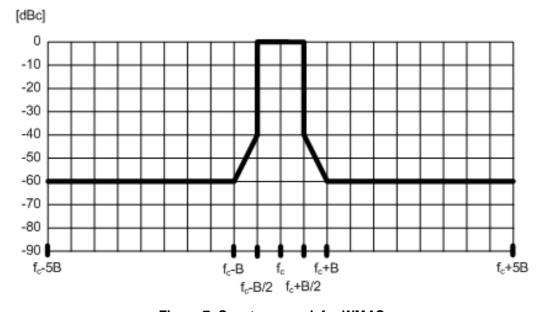
Figure 7: Spectrum mask for WMAS
