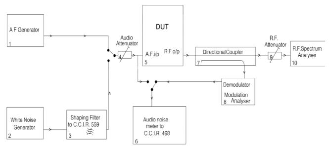
NOTE: If the DUT incorporates ancillary coding or signalling channels, for example, pilot tone, etc. these should be switched on prior to measuring the transmitter RF output spectrum.
