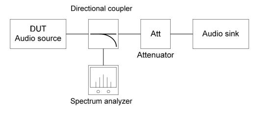
Figure 6: Measurement setup for WMAS
