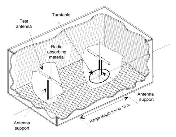
Figure C.1: A typical anechoic chamber
