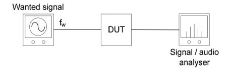
Figure 10: Measurement setup for Rx sensitivity
