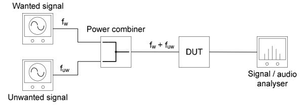
Figure 11: Measurement setup for receiver adjacent channel selectivity
