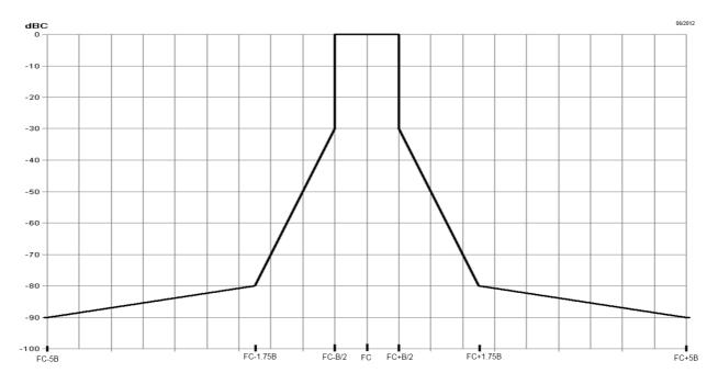
Figure 4: Spectrum mask for digital systems below 2 GHz
