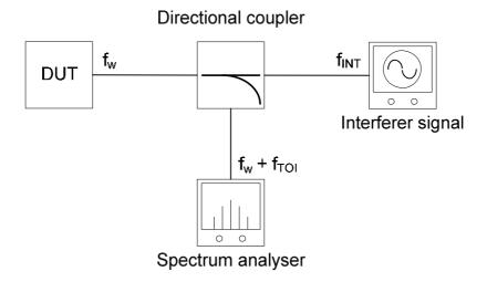
Figure 9: Measurement setup for Tx-IMD
