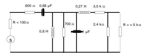
Figure 2: Filter circuit
