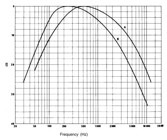
NOTE 1: Curve A = Frequency spectrum of standardized noise (measured with one-third octave filters).
