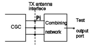
Figure B.2: Transmitter test set-up
