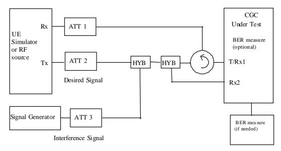
Figure D.5: Measuring system Set-up for Blocking characteristics
