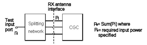
Figure B.1: Receiver test set-up
