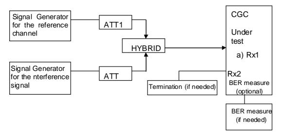
Figure D.4: Measuring system Set-up for Adjacent channel selectivity
